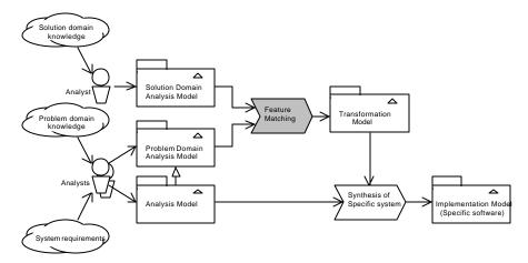
Figure 3. Model-based software engineering process with feature matching
